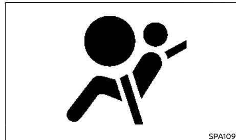
The supplemental air bag warning light, displaying
