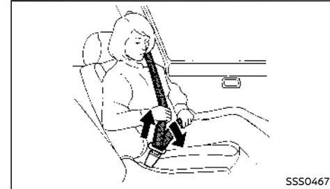
3. Position the lap belt portion low and snug on the hips as shown.
