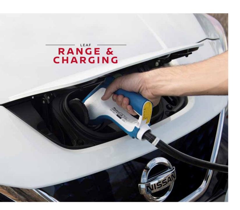
When the first generation Nissan LEAF arrived in Australia in June 2012, the then 24kWh laminated lithium-ion battery gave owners a NEDC driving range of 170kms.
